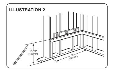
**D.)** Install drain components to the bath following the manufacturer's instructions. See the roughing-in drawing for suggested opening size and location dimensions.
